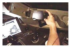
Unfold the chart holder to open it into a flat platform.
