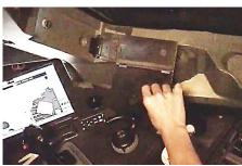
Hold the PIVOT LTRM in one hand and slide it onto the chart holder.
