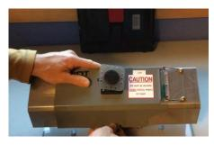
Lift the chart spring clip push the unit forward until the raised tab on the LTRM is captured by the chart spring clip.
