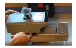
Lower the LTRM onto the shroud and rotate it slightly forward toward the chart spring clip.
