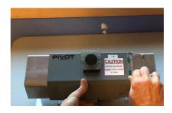
Pull inward on the tab in the center of the LTRM to clear the bottom of the window shroud.
