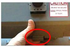
Lift upward until the LTRM pops off the window shroud.
