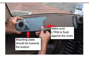
Hold the arm which the mounting plate is secured to and push to slide the entire LTRM forward.
