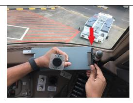
With the other hand, lift up on the lower edge of the LTRM to remove it from the chart clipboard.
