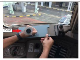
As the LTRM slides towards the top of the table, lift the chart spring clip to allow the LTRM to sit flush against the top of the chart table.
