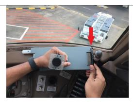
Release the spring clip, ensure the spring clip sits outside the raised detent of the LTRM to ensure the LTRM stays firmly in place.
