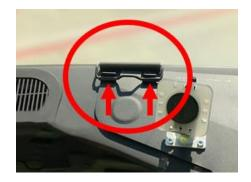
Lift the forward chart spring clip up and over the vertical tabs on the LTRM. Slide the LTRM out from underneath the raised clip. Then lower the clip.
