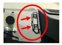
Raise the aft/outboard chart spring clip. Rotate the LTRM so the outboard edge of the LTRM abuts the raised clip housing. Lower the clip to capture the 2 vertical tabs on the LTRM.
