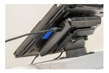
STEP 2: Press the PIVOT Clip to disconnect the PIVOT case from the mounting plate and slide the tablet to the side to remove it from the DKS adapter.
