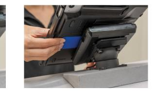
The PIVOT DKS Adapter does not need to be removed from the Thales DocKing Station. We suggest you leave the adapter in place on the aircraft. However, if removal is desired, press the tab on the DocKing station (ADKS) and slide up to remove the DKS adapter from the ADKS DocKing station.
